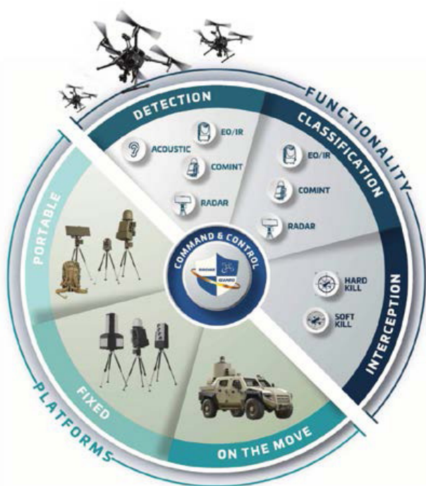
Fig.5: Concept modern C-UAS ELI 4030 (sursa: https://www.iai.co.il/p/eli-4030-drone-guard#gscw504792 , accesat la 06.02.2025)
